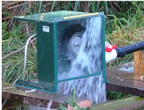
Running slow – water exhausting towards jet
