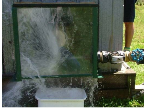
Running too fast, exhaust water hits other side of casing
